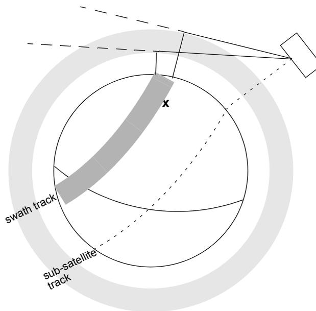
**Figure 5 Limb-sounding instrument: swath definition (2)**
