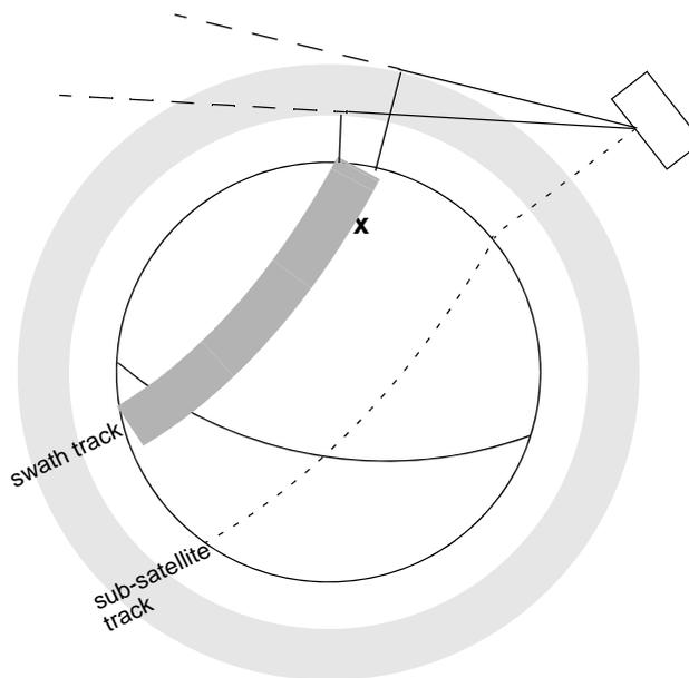
**Figure 5 Limb-sounding instrument: swath definition (2)**
