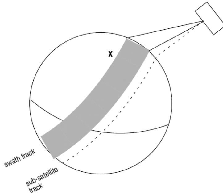
**Figure 15: Earth-observing instrument: swath definition**
