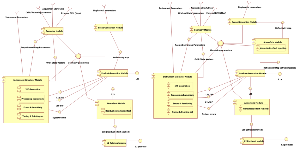
Figure 9-9: Component diagram for the reference architecture including residual atmospheric effects injection, on the left, and for the reference architecture including atmospheric effects injection and atmospheric effects removal, on the right.
