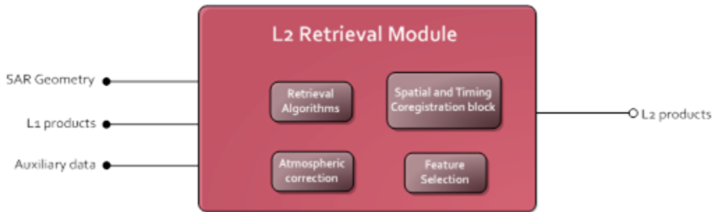
Figure 9-24: Input and output interfaces of the Level 2 Retrieval Module
